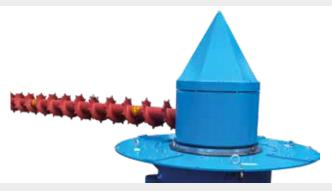
Sturdy construction to take in extremely high feed loads when discharging from high silos. Especially designed for shavings and large diameter bunkers.
