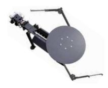
For discharge of fuels from bunkers with a maximum working diameter of 6 metres. The system is low maintenance and is especially designed for fuels with increased discharged output due to their limited ability to flow. The patented design guarantees quiet and effective operation. The feed screw with progressive screw blade ensures low energy consumption.
