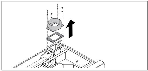
$\ensuremath{\square}$  Unscrew the four hexagon bolts and remove the flue gas pipe nozzle with the seal
