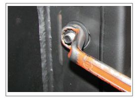
Loosen the lock nuts at the top and bottom of the locking plate using an Allen key (13 mm)
