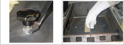
Remove the heat exchanger cover and combustion chamber cover to further reduce the weight
