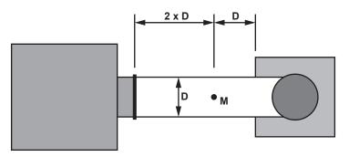
In front of the measuring port (M) a straight inlet section should be located at a distance corresponding to about twice the diameter (D) of the connecting piece. A straight outlet section at a distance corresponding to about the single diameter of the connecting piece should be provided after the measuring port. The measuring port must remain closed whenever the system is in operation.
