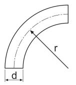
The ratio of the radius of curvature (r) to pipe diameter (d) should be greater than 1 r:d  $\geq 1$
