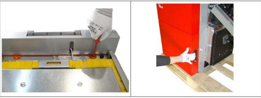
□ Remove the two screws and contact washers from the flaps of the controller cover Caution: Do not lose the contact washers! □ Open the insulated door (P4 Pellet 15/20/25)
