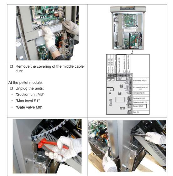
$\ensuremath{\square}$  Undo the cable ties at the cable leadthrough
