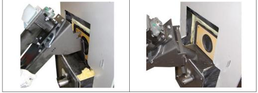
$\hfill\square$  Pull the stoker unit up slightly until the hooks come out of the stoker flange
