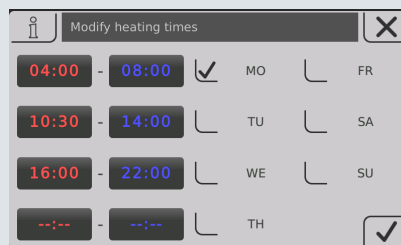
Fig. 2 View of the heating times (individually adjustable)
